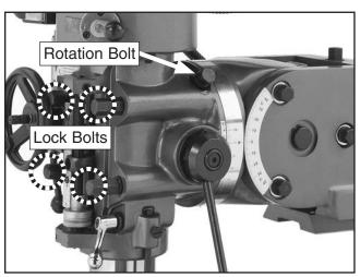
Figure 23. Head rotation controls.
